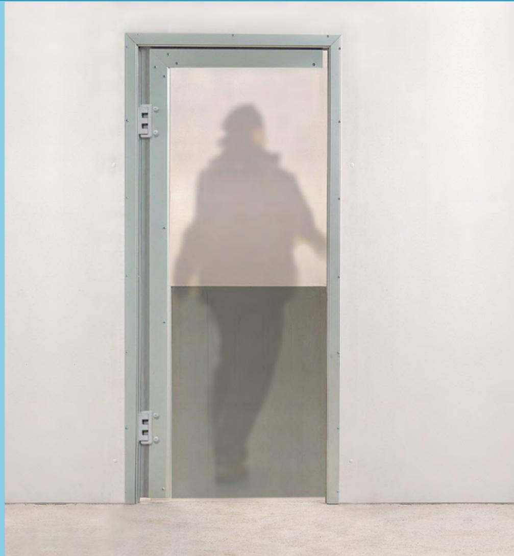
The PK double action hinged high visibility doorset consists of a 5 mm thick clear food grade polycarbonate doorleaf supported by an aluminium reinforcement channel along the hinge and top edge. This is hung on a fully adjustable aluminium wrap around frame system. The doorleaf is flexible, lightweight and durable. Designed to provide maximum visibility in high traffic areas. Can be fitted to brick or block openings and most other wall materials.
